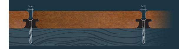
Hidden fastener clips are a great way to secure your deck without screwing into the board's face. Our Kebony Deck Board is compatible with the Fastenator™ Hidden Fastening system by DuraLife®.
