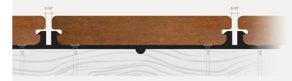
Step-Clip<sup>TM</sup> for Kebony uses easy to install strips to minimize the time and labor spent fastening your deck. The Step-Clip reduces deck surface installation time by up to 50% and ensures proper spacing, protects the joist from water damage, and makes it easy to replace a board in the future if necessary.
